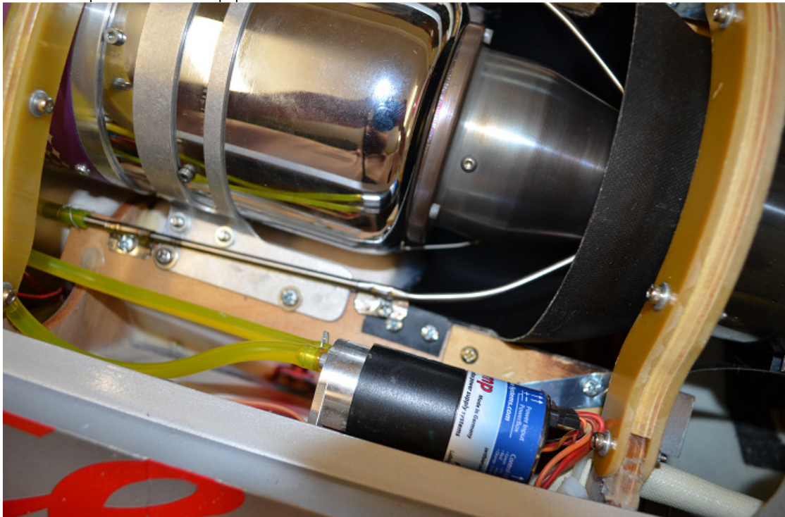
Photo 6 – position of aft pipe
