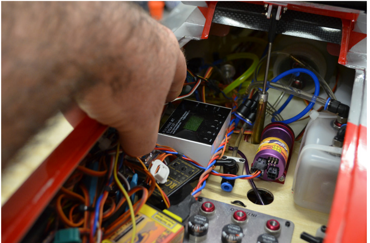
Photo 3 – sample layout of air systems on forward component board. Leave room for cockpit above
